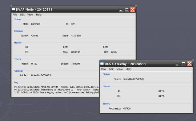
The G4KLX Repeater software provides the building blocks for making your own analogue (FM) and D-Star repeater systems — this is gateway onto the DCS reflector system using a DV Access Point Dongle...
